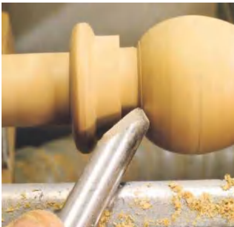
▲ Pic.22 The bottom or swell on the ogee shape is turned once again with the gouge; the bevel rubs as the tool is moved to the left. You can see that the flute of the tool is completely closed at the end of the cut
